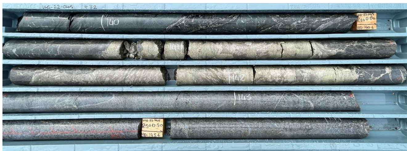
Figure 3. Massive and matrix textured nickel intercept in underground diamond drilling, LN04a (ULG-22-045)
