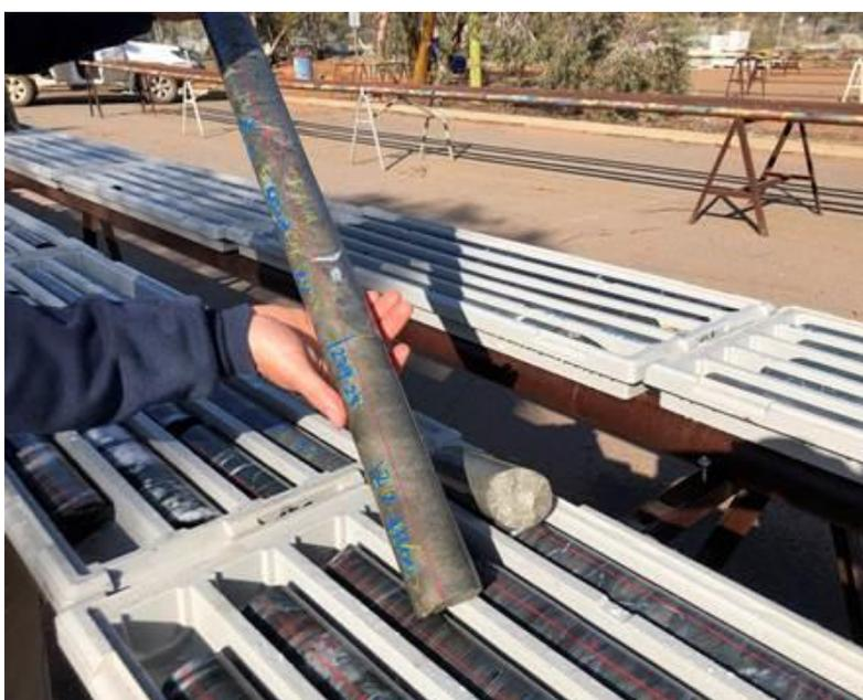
Figure 2: Close-up of MDD350 massive nickel sulphides
