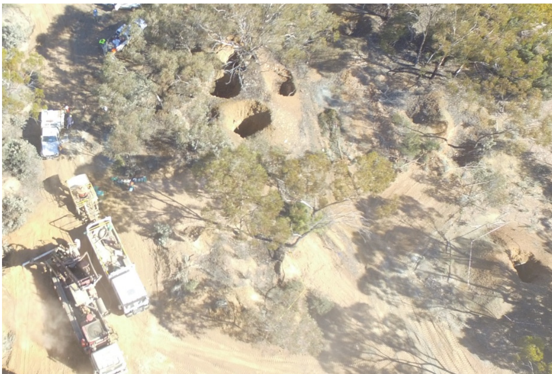
FIGURE 1: RC Drilling around the numerous artisanal shafts accessing various gold lodes at the Flinders Project
