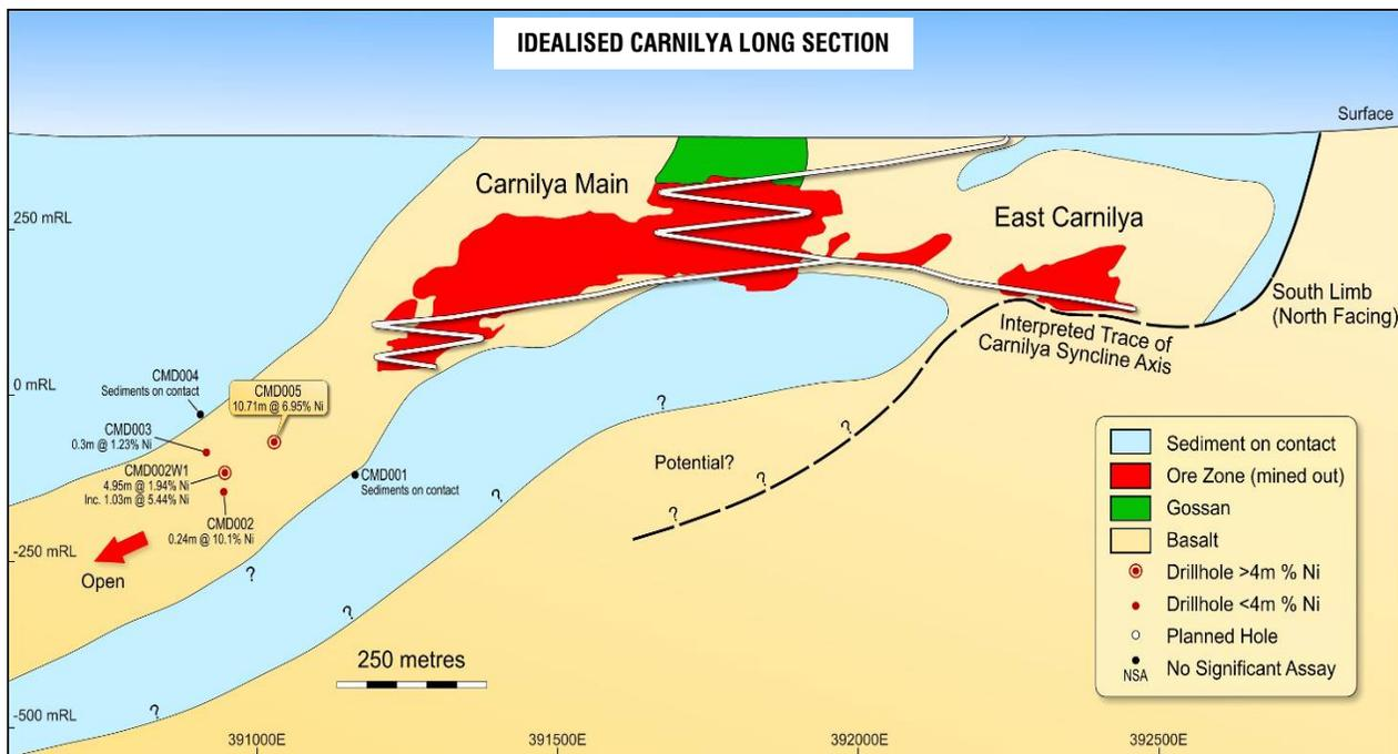
DHEM surveying of CMD002 indicated a significant conductor up-dip, and a wedge was drilled from this parent hole. CMD002W1 intersected the contact approximately 35 metres up-dip of the original intersection and returned **4.95 metres @ 1.94% nickel** from 590.91 metres, including **1.03 metres @ 5.44% nickel** from 591.02 metres depth, in matrix and disseminated sulphides. Both intersections are close to true widths.
