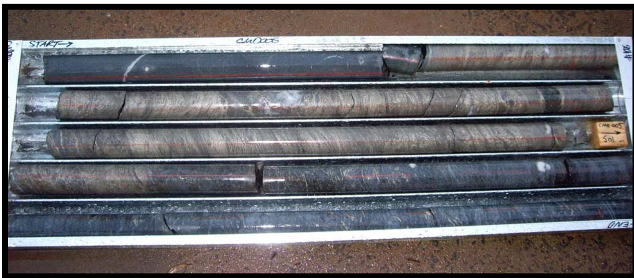
Photograph of massive nickel sulphide mineralisation in drill hole CMD005 at Carnilya Hill, grading over 11% nickel, part of a wider intersection of 11 metres @ 6.95% nickel.
